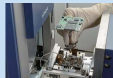
Accommodates samples of sizes up to 70 mm (diameter) x 50 mm (thickness) * We recommend using gloves to prevent contamination.
